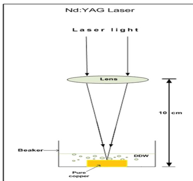
**FIGURE 1.** Schematic diagram of PLAL system.
