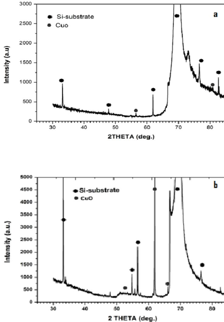
FIGURE 4. XRD spectrum of nanoparticles CuO/Si synthesized by laser ablation at (a) 150 mJ/puls and (b) 300 mJ/puls.
