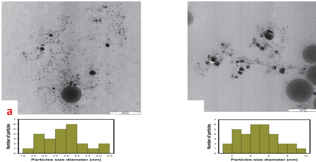
**FIGURE 3.** TEM images and sizes distribution of the CuO nanoparticles produced by laser energy at (a) 150 mJ/puls and (b) 300 mJ/puls.
