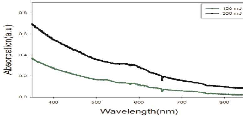
**FIGURE 2.** UV/Vis spectra of the colloidal dispersion containing particles synthesized by laser ablation of Cu target at 150mJ/puls and 300mJ/puls
